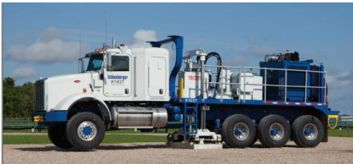
Figure 2. Schlumberger Vibroseis Unit
